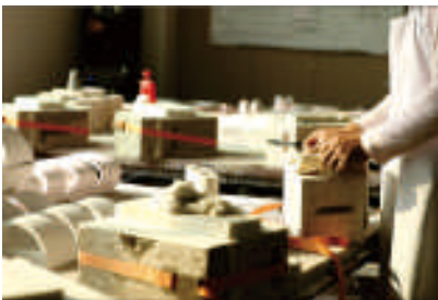
Step 05: Demoulding Molding
